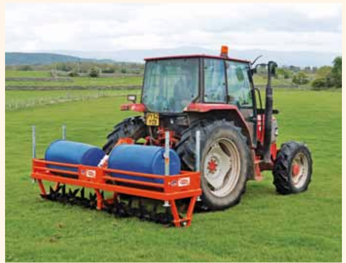
Soil Aerator from the Eden River Trust which farmers can borrow to trial soil aeration to reduce rapid run off from farmland during rainfall Source: Eden Rivers Trust, UK
